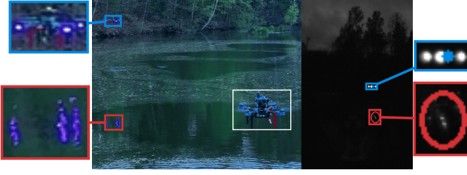
Fig. 7: Outdoor experiment: (Left) Observing UAV (white), transmitting UAV with active markers (blue), and surface reflections (red). (Right) Onboard UV-filtered image showing the detected marker centroid (blue) and reflection ellipse (red).
